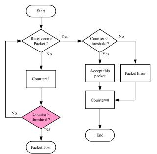
Figure 4. Flowchart of Packet loss detection
